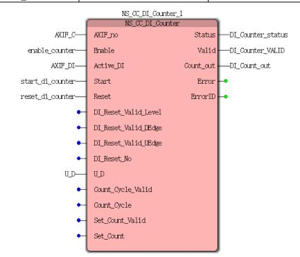
**Case 1:**When enable\_counter from FALSE to TRUE, and held, start\_di\_counter start permission from FALSE to TRUE DI-speed counter, DI\_Count\_out display the current count of pulses. When reset\_di\_counter a FALSE to TRUE, Count\_out display the current pulse count value is 0, then the count pulse input DI, Count\_out display the current pulse count remains at 0 when the Reset TRUE to FALSE, allowing counting resumes .
