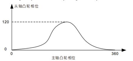
When the main shaft when both the absolute mode, and performs the engagement operation, the main are 0, and scaling without using the offset from the position of the shaft axis (the default), the main execution of the real position of the cam shaft corresponding relationship As shown below:
