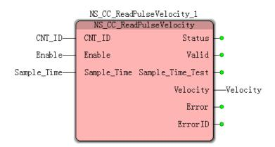
**Case 1:**In the servo axis operation when the Enable FALSE to TRUE, the output module Velocity servo axis current operating speed, if you want to interrupt the conversion speed consistent actuator need to be converted according to the above formula.
