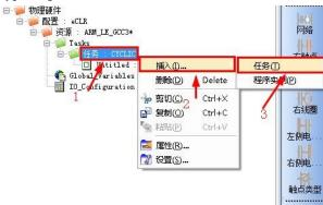
Step 6: New "Task Type" right "Tasks" click "insert", and then select the "Tasks" as shown.
