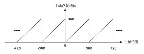
When SlaveAbsolute parameter is TRUE, the position of the shaft between the shaft and its absolute cam phase relationship, at any time, from the phase of the cam shaft is equal to the time to make the position of the cam shaft from a relationship between the shaft axis from a maximum range value modulo result of the operation. When the absolute mode Slave axis, consistent with the correspondence relationship between the phase of its spindle axis position and its cam.
