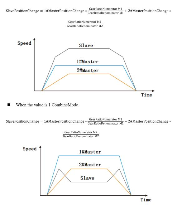
Mainshaft gear ratio numerator and denominator are adjusted to set the amount of change of the two spindle positions factor using Equation supra.
