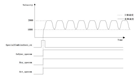
• Spindle speed 1000, execution NS\_MC\_SpecialCombineAxes, made in accordance with the motion from the shaft of the cam follower shaft position change table.
