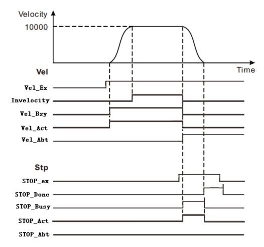
• When Vel\_Ex becomes TRUE, after a period Vel\_Bsy, Vel\_Act becomes TRUE, the servo motor begins to move forward. When the servo motor reaches the target speed, Invelocity becomes TRUE.
