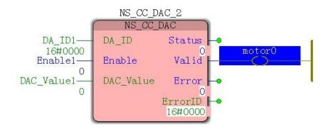
(4) the online debugging mode, when the Enable becomes FALSE TRUE by the (already in ensuring the servo enabled state), if the motor is running at the speed of zero drift, DAC\_Value adjustment value at this time to ensure that the servo drive in a stationary state, Enable the TRUE to FALSE, offset adjustment is completed, and then completing the axis parameters as the initial value of the value DAC\_Value MC\_AXIS\_REF (axis parameter) of the module Middle\_Value.
