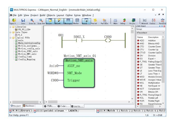
Step 3: In the user-defined library, find the "M otion\_NMT\_axis" block, hold down the left mouse button and drag it to the programming interface, then let go, then the module's properties will pop up, you need to name the module, generally keep the default., click "OK", as shown below;
