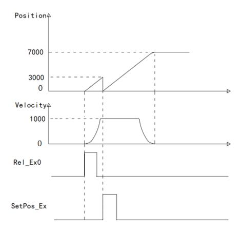
• MC\_ReadActualPosition execution instruction fetch real-time position, the MC\_MoveRelative performed, charged at a set speed to the target shaft position 10000
