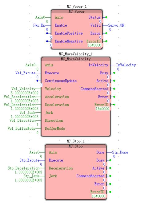
Debug 1: Double-click the input function bit Pwr\_En to pop up the debug: Resource interface, select the value of the variable Ture, then click overwrite, Pwr\_En will change from False to Ture, as shown in the figure;
