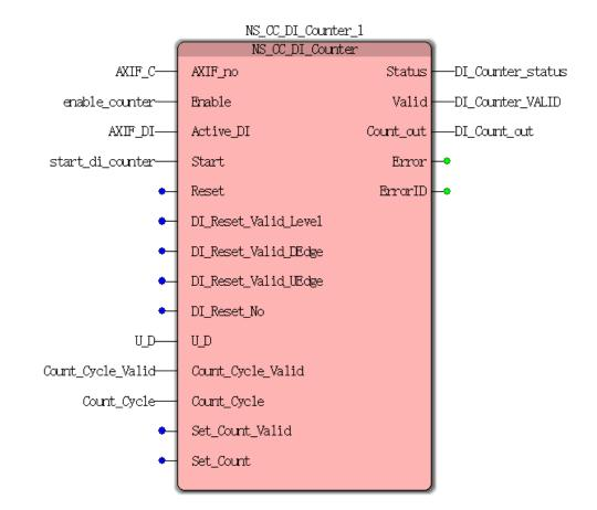
**Case 1:**When enable\_counter from FALSE to TRUE, and held, start\_di\_counter start permission from FALSE to TRUE DI-speed counter, a pulse to DI11, DI\_Count\_out display the current pulse count is incremented, up to 1000 when DI\_Count\_out recounting is automatically cleared.
