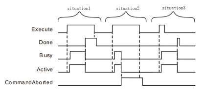
**Case 1:**When the Execute FALSE to TRUE, after a period, Busy, Active becomes TRUE. When you have two spindles and synchronous slave axis, InSync becomes TRUE, while Busy Active and remains to TRUE.
