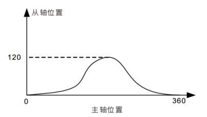
When the position of the offset or scale is not the default value, as the corresponding impact relations from the actual position of the main cam execution:
