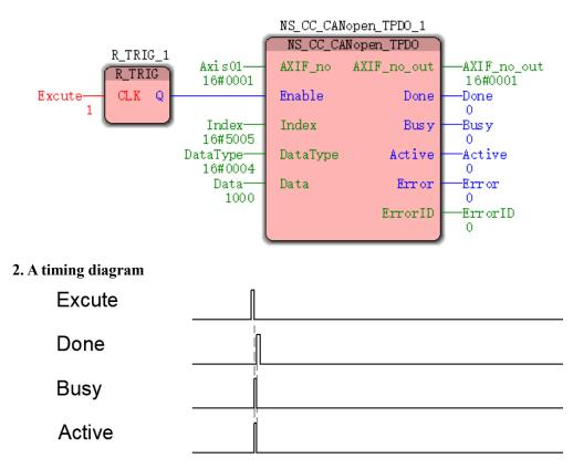
As shown, 0X60FF RPDO mapping data mapping area, index 0X5005 (custom master station), then the "Index = 16 # 5005", due to DINT 0X60FF type, the "DataType = 16 # 04", "Data = 1000"1000 will be assigned to the trigger module node address 0X60FF, it indicates that the current node profile speed setting value is set to 1000.
