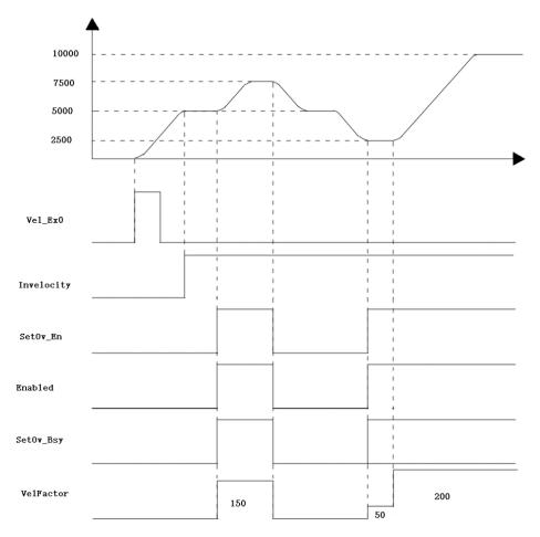
• When Vel\_Ex0Becomes TRUEAfter time, a period Vel\_BsyAnd Vel\_Act becomes TRUEAfter axis starts forward rotation, the output reaches the set speed Invelocity TRUEAnd then SetOv\_EnSet TRUEWhile Enbaled, SetOv\_BsyBecomes TRUE, MC\_SetOverride effective date of the controlled axis according VelFactorThe value of re-generate the target speed.
