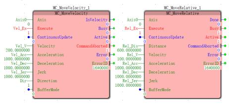
Debug 3 : At this point, double-click Stp \_Ex to change its value from False to True, and the controller will control Axis 0 anDAxis 1 to decelerate according to the set deceleration until it stops, as shown.
