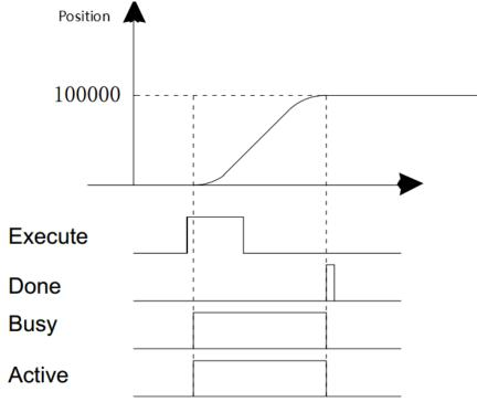
• When the Rel\_Ex FALSE to TRUE, a period, while the Busy and Active is TRUE, starts executing the instruction in accordance with the relative displacement of the parameter setting, the current position of the axis at this time is 0, the target location is 100,000.
