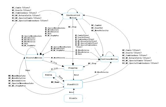
Note1: Enable with MC\_Power command and MC\_Power. Status is True. Note2: MC\_Stop.Done is True and MC\_Stop.Execute is False.
