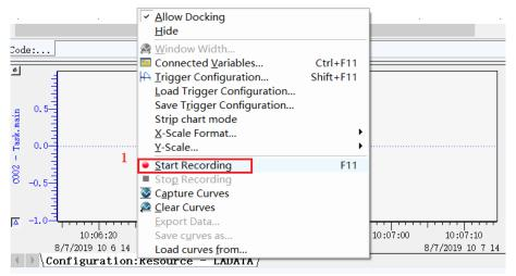
6) Note that when you click "Start Recording", try not to perform other operations. Otherwise, the communication will not be smooth or crash. If you want to perform other operations, stop the recorder first and then perform other operations. The final monitoring result is as follows: The figure shows. To stop monitoring, repeat the fifth operation and select "Stop Recording".
