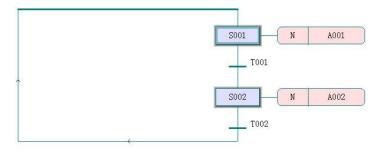
(4) Click " Step " S002, then click " Insert SFC Branch ", then insert a branch on the right side of " Step " S002, the branch has a " Step " S002, as shown
