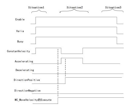
Case 1: In the controlled axis is Standstill state, when the Enable from FALSE to TRUE, and Busy vaild simultaneously become TRUE, ConstantVelocity, Accelerating, Decelerating, DirectionPositive, according to the output pin axis DirectionNegative state to TRUE or FALSE.
