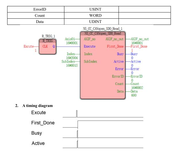
As shown, the servo read parameter P04.21 Vector (the current rotation speed, the unit r / min), the corresponding index: 2000 + # 16 # 16 16 # 4 = 2004, corresponding to the sub-index 21 16 # 15, the trigger module No. 1 reads the current speed of the servo node 600r / min.
