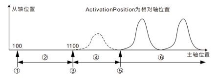
stage ①: Trigger MC\_CamIn instruction is executed, this time to the absolute position of the spindle 100
