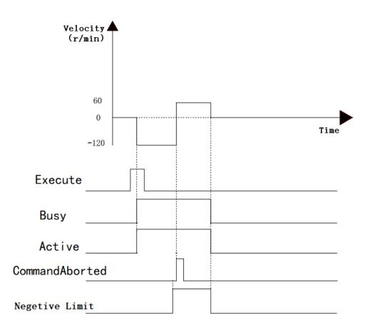
• Mode = 17, when the Home\_Ex becomes FALSE TRUE, the motion controller controls the operation of the servo motor, means starts reverse rotation, after reaching the reverse limit switch is turned forward, and then leaving the stop position of the reverse limit switch, so as to drive institutions back to the mechanical origin position A.
