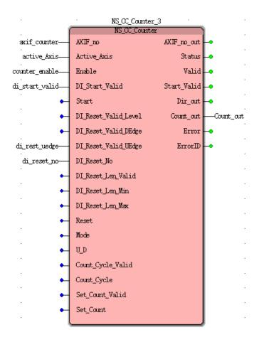
**Case 1:**When counter\_enable FALSE to TRUE grounds, and maintained. di\_start\_Valid becomes TRUE, and if the external signal DI3 signal is valid, the counter 3 starts counting the number of high, Count\_out display the current pulse when the rising edge DI0 di\_reset\_no specified, the current value of the high-speed counter is cleared.
