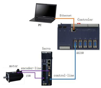
According to the above system , the servo motor is controlled to start, run and stop by the motion controller.
