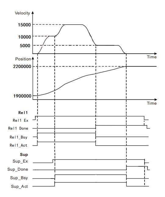
• When Rel\_Ex becomes TRUE, after a period Rel\_Act, Rel\_BsyBecomes TRUE, the motion controller controls the operation of the servo motor to the current position as a reference point.
