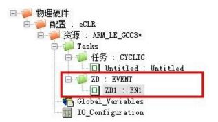
**Step 12:** "Project" Return "Project Tree Window" in the window, double-EN1 at POU join a summing module (purpose is to verify whether the interrupt routine is executed correctly)
