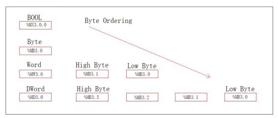
Such as: a hexadecimal number stored in 16% MW3.0 # 1234 in the presence of 16% MB3.0 # 34, the # 12 is stored in 16% MB3.1 in. If the procedure for bit operations, it will affect the place where the byte, word and double-word and vice versa.
