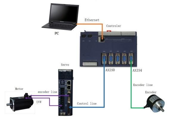
According to the above system, the control servo motor runs an electronic gear following the spindle (encoder);
