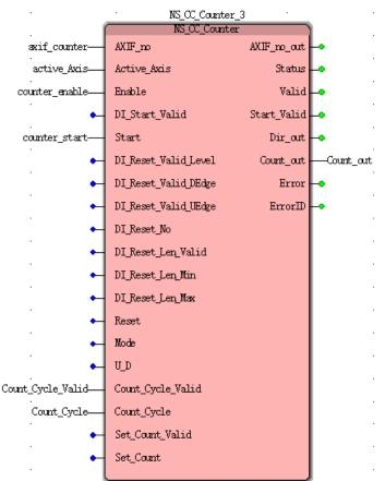
**Case 1:**When counter\_enable from FALSE to TRUE, and held, counter\_start from FALSE to TRUE starts allows high-speed counter, Count\_out display the current count of pulses. When the high-speed counter current value of 5000, the counter is automatically cleared recount, constant cycle.
