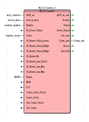
**Case 1:**When counter\_enable from FALSE to TRUE, and held, counter\_start from FALSE to TRUE starts allows high-speed counter, Count\_out display the current count of pulses. When the RESET FALSE to TRUE, Count\_out display the current pulse count is 0, then the number of the input pulse, Count\_out display the current pulse count remains at 0 when the RESET TRUE to FALSE, allowed to continue to start counting.
