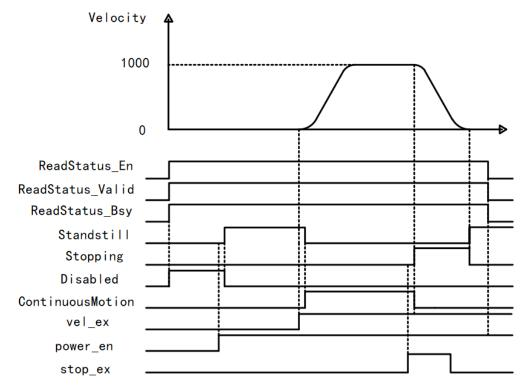
• Enable MC\_Power from FALSE to TRUE instruction, the latter instruction cycle Disabled MC\_ReadStatus by TRUE to FALSE, while Standstill MC\_ReadStatus instruction from FALSE to TRUE (i.e., the state machine changes from the Disabled Standstill)
