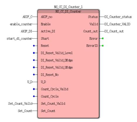
**Case 1:**When counter\_enable a FALSE to TRUE, start\_di\_counter start permission from FALSE to TRUE DI-speed counter, DI\_Count\_out display the current count of pulses. When the change from FALSE to TRUE Set\_Count\_Valid variable, high-speed counter current value be modified Count\_out 1000, and 1000 remain, a TRUE when Set\_Count\_Valid variable becomes FALSE when DI11 pulse is received, will continue to count the number of pulses on the basis of 1000 increments.
