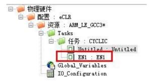
**Step 5:** Select under "Project Tree Window", "Hardware", under Resources "task", rightdelete "EN1" program and click "OK" we need another new "task type", as shown below.
