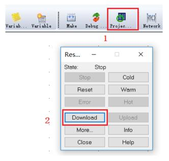
2) After the program "Download" is completed, click the "Cold Start" program on the resource panel to run, and the status display "Run" indicates that the user program is continuously looping; the user can debug online, monitor the status of the variable, click "Debugging on " on the toolbar, Screen effect during simulation, as shown.
