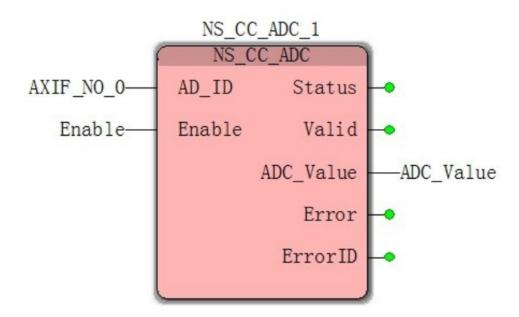
Case 1: When the Enable FALSE to TRUE, the external input AI0 DC5V, the controller converts the 5V voltage into a digital output displays ADC\_Vable 3070 (there may be errors to the actual subject)
