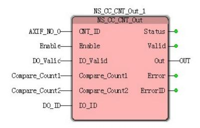
**Case 1:**Start NS\_CC\_Counter\_1 (high-speed counter module), when the Enable FALSE to TRUE, the execution instruction module, when the current value of the pulse high-speed counter at 1000 and 5000, Q0.0 will output, OUT will be FALSE to TRUE, the current pulse values outside 1000 and 5000, Q0.0 is not output, OUT by TRUE to FALSE.
