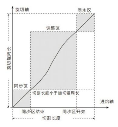
When feeding short cut, peeling axis adjustment must be accelerated in the region, and then decelerate to synchronous speed.
