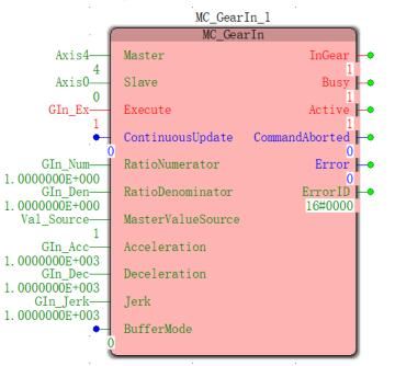
Commissioning 3 : At this point, turn the spindle (encoder) and the slave axis (servo axis) will follow the spindle in accordance with the 1: 1 electronic gear ratio.
