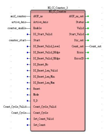
Case 1:When counter\_enable a FALSE to TRUE, counter\_start from FALSE to TRUE starts allows high-speed counter, Count\_out display the current count of pulses. When
