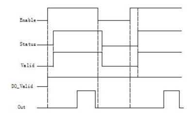
**Case 1:**When the Enable FALSE to TRUE, Status Valid and becomes TRUE after a period and, FALSE when Enable changed from TRUE, Status Valid and from FALSE to TRUE and after a cycle.
