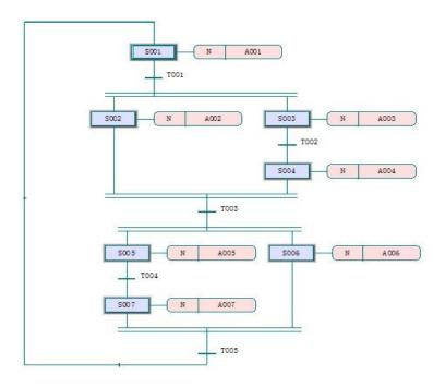
At this point, aNSFC network is created, in which S001 is the initial step, the user can use the initialization data, such as the counter to clear the initial value and other operations, and then according to the requirements of the "step", "conversion" to write code and The setting of the property.
