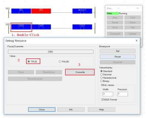
3 Select the radio button "TRUE" and click on the "Force" result, the variable will be forced to "ON" and will be highlighted in red on the online work order.
