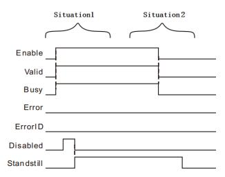
Case 1: When the Enable FALSE to TRUE, Vaild Busy and simultaneously become TRUE, ErrorStop, Disabled, Stopping, Homing, Standstill, DiscreteMotion, ContinuousMotion The shaft and SyncMotion state to TRUE or FALSE.
