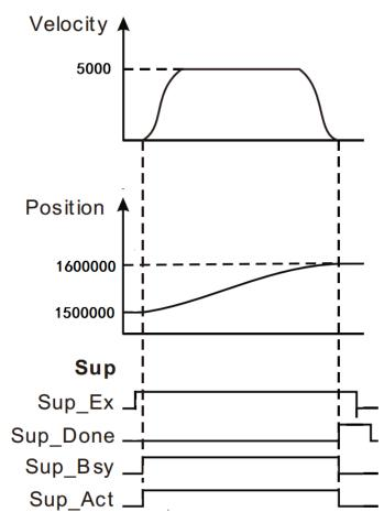
• When Sup\_Ex becomes TRUE, after a period, Sup\_Bsy, Sup\_Act becomes TRUE, the motion controller controls the operation of the servo motor to the current position as a reference point.
