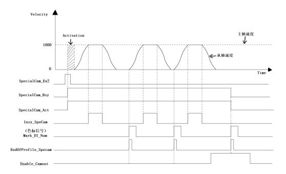
Mode = 1 NS\_MC\_SpecialCamIn to execute instructions, the Execute becomes TRUE, after a period, Busy, Active becomes TRUE, in this case as a starting point, when the spindle reaches the Activation, the distance Slave axis in accordance with the acceleration set to sync area in the sync area inner, InSync output TRUE, and then completes the synchronization deceleration distance from the end of the first synchronization period.
