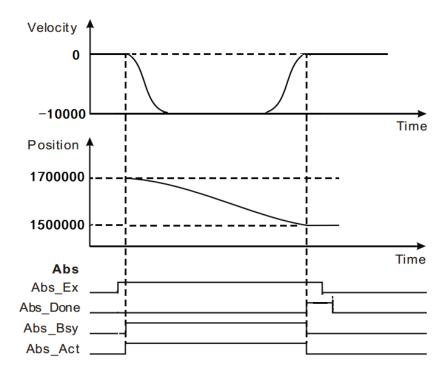
• When the Abs\_Ex MC\_MoveAbsolute FALSE to TRUE to start the instruction execution, the current position of the axis at this time is 1.7 million, 1.5 million target position.
