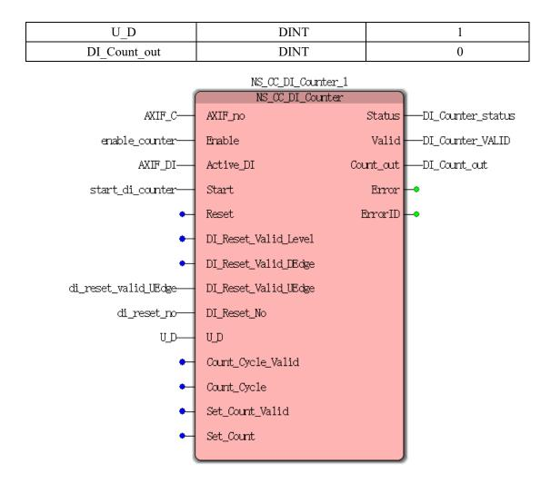
**Case 1:**When enable\_counter from FALSE to TRUE, and held, start\_di\_counter start permission from FALSE to TRUE DI-speed counter, DI\_Count\_out display the current count of pulses. When the rising edge of DI di\_reset\_no specified, Count\_out current pulse count value is cleared.
