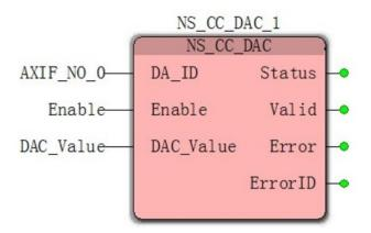
situation1: When Enable changes from FALSE to TRUE, Valid changes from FALSE to TRUE, and the next cycle, the analog quantity output 0V, the modified variable DAC\_Value is 1024, the analog output 5V.
