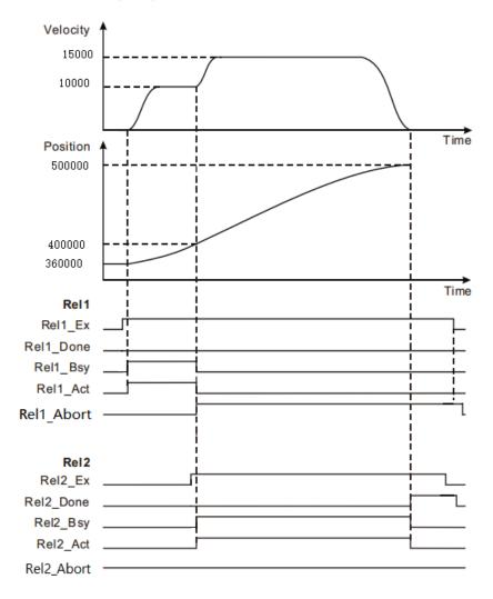
• When Rel1\_Ex a FALSE to TRUE, the first MC\_MoveRelative instruction starts execution, the current position of the axis at this time is 360 000, the position of the target
