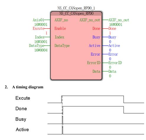
As shown, 0X60FF TPDO mapping data mapping area, the index 0x5001 (master defined), then the "Index = 16 # 5001", Type "DataType" is defined as follows:
