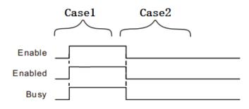
Case 1: When Enable the FALSE to TRUE, Busy, Enabled To TRUE
