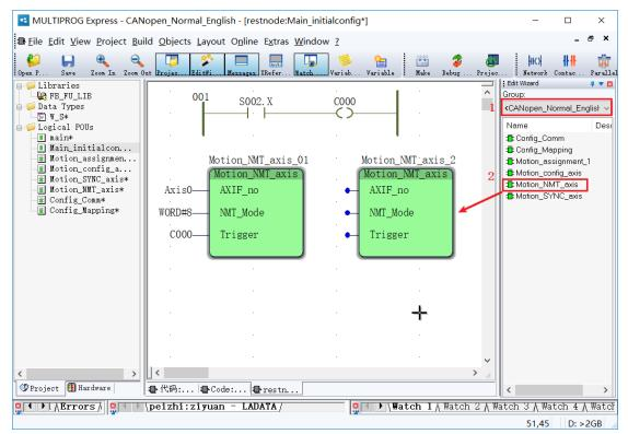
Step 4: Double-click the module input pin (blue dot), and the "Variable Properties" box
