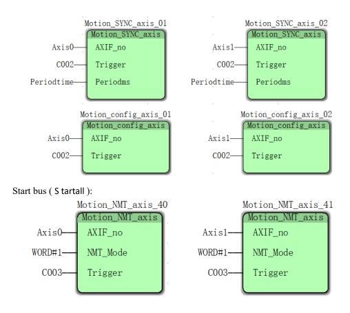
Step 6: After completing all the process configuration, click on the production and confirm that it is correct. At this point, the CANopen communication configuration of node 2 (Axis 1) has been completed;
