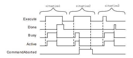
**Case 1:**When the Execute FALSE to TRUE, Busy and Active simultaneously become TRUE. When the positioning is completed, Done becomes TRUE, and the Busy Active becomes FALSE, if after the completion of the positioning, Execute a TRUE to FALSE, after a period, Done becomes FALSE.
