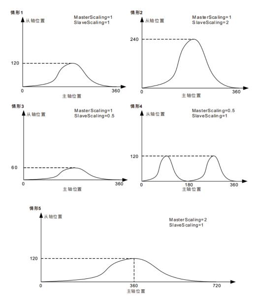
**Case 1:**When the main shaft from the zoom ratio is 1, the offset is zero, consistent with the actual relationship between the cam and the pre-planned.
