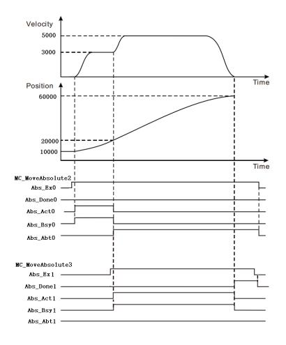
• When Abs\_Ex0 a FALSE to TRUE, the first MC\_MoveAbsolute instruction starts execution, the current position of the axis at this time is 1000, the target location 3000.
