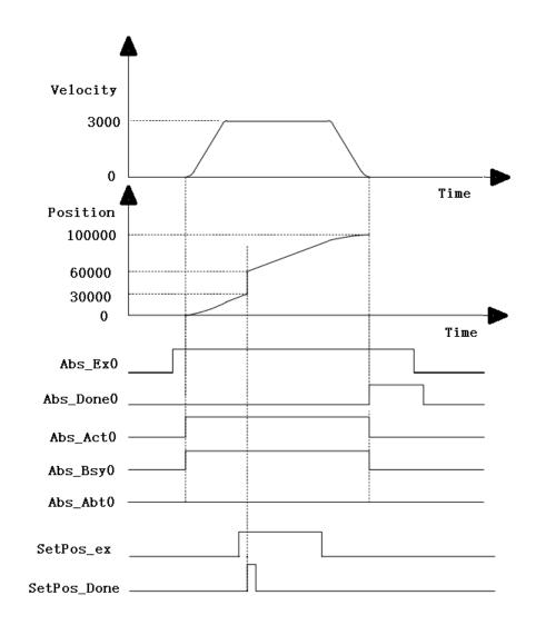
• When Abs\_Ex0 a FALSE to TRUE, MC\_MoveAbsolute instruction starts execution, MC\_SetPosition instruction execution when the current position is greater than 30,000.
