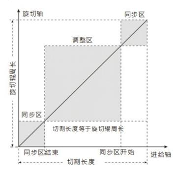
In this case, sync area with the non-synchronous zone peeling axis and the feed axis speed synchronization has been maintained, no adjustment peeling axis.
