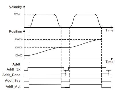
• When Addt\_Ex a FALSE to TRUE, the motion controller controls the operation of the servo motor to the current position as a reference point, after a period Addt\_Bsy, Addt\_Act becomes TRUE. After the completion of the servo motor set distance, a done bit Addt\_Done FALSE to TRUE, and at the same time Addt\_Bsy Addt\_Act a TRUE to FALSE.
