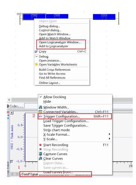
4) In the pop up "trigger Configuration" "check" continuous recording, and click " OK ", shown in FIG.
