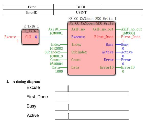
When the above, the servo parameter assignment Vector P03.19 (position error value is too large), the corresponding index: 2000 + # 16 # 16 16 # 3 = 2004, corresponding to the sub-index 19 16 # 13, a length of 4 bytes, the current No. 1 trigger module assignment node position is too large value.
