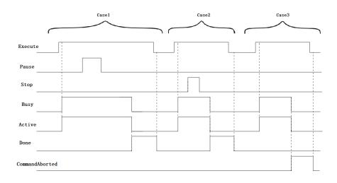
**Case 1:**When the Execute FALSE to TRUE, after a period, and Busy Active simultaneously become TRUE, during execution of instructions, a Pause FALSE to TRUE, the operation of the pause instruction is executed, but still Busy Active TRUE and, when changed from TRUE Pause after it is FALSE, the controlled shaft work to finish the operation. When the instruction is complete, Busy and Active becomes FALSE, while Done becomes TRUE. After the Execute cycle by TRUE to FALSE, Done becomes FALSE.
