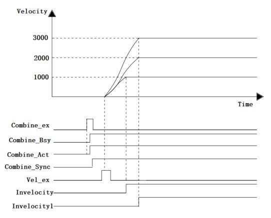
• When the Combine\_ex FALSE to TRUE, MC\_CombineAxes instruction starts execution, after some time, the instruction is executed successfully, Combine\_InSync becomes TRUE, the three axes in accordance with the instruction required to achieve synchronous movement
