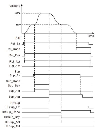
• When Rel\_Ex becomes TRUE, after a period, Rel\_Bsy and Rel\_Act becomes TRUE, the motion controller controls the operation of the servo motor to the current position as a reference point. Sup\_Ex becomes TRUE when, after a period, Sup\_Bsy and Sup\_Act becomes TRUE, MC\_MoveSuperimposed instruction starts execution, and an acceleration of the servo motor speed will (in this case acceleration is 0 axis) is superimposed.
