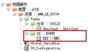
**Step 11:** "Project" Return "Project Tree Window" in the window, double-EN1 at POU join a summing module (purpose is to verify whether the interrupt routine is executed correctly)
