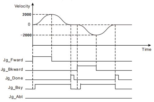
When the Jog\_Forward NS\_MC\_Jog FALSE to TRUE to start execution instruction, after a period of Jog\_Bsy FALSE to TRUE, the axis movement in positive direction; FALSE to TRUE to the Jog Forward, the shaft begins to decelerate, when the deceleration is 0, Jog Bsy
