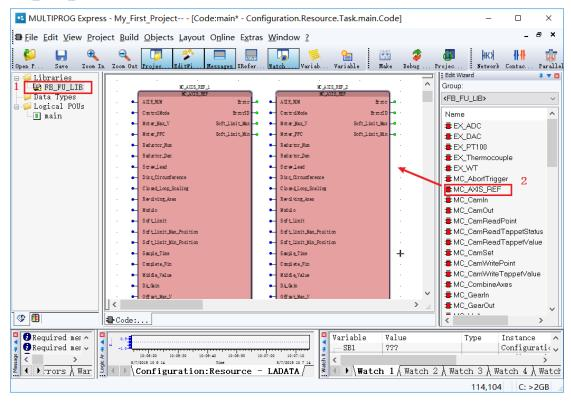
Step 2: Double-click the module input pin (blue dot), and the "Variable Properties" box will pop up to define the variable name, data type, usage, initial value, etc., as shown in the figure ;
