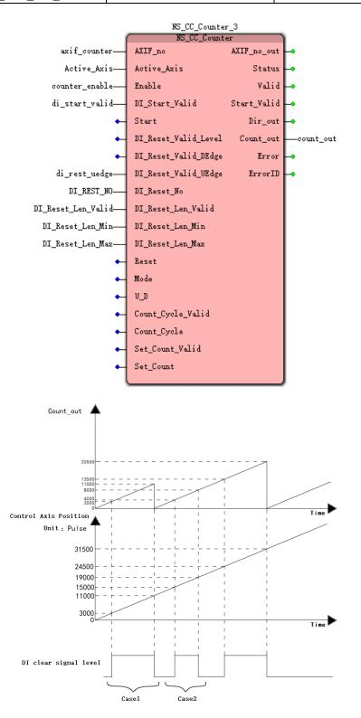
**Case 1:**When counter\_enable FALSE to TRUE grounds, and maintained. di\_start\_Valid becomes TRUE when the external signal DI3 signal is valid, the counter 3 starts counting the number of high, Count\_out display the current pulse, when the designated DI0 di\_reset\_no from FALSE to TRUE again until DI0 becomes FALSE, the controlled axis through this period
