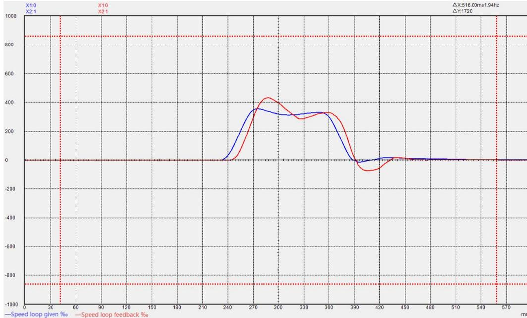
If the integral gain of the speed loop is too small, the rigidity of the motor is very weak and the speed cannot follow.
