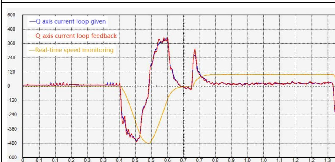
The Q-axis current has low frequency oscillation, and it is necessary to reduce the current loop integral gain P07.02
