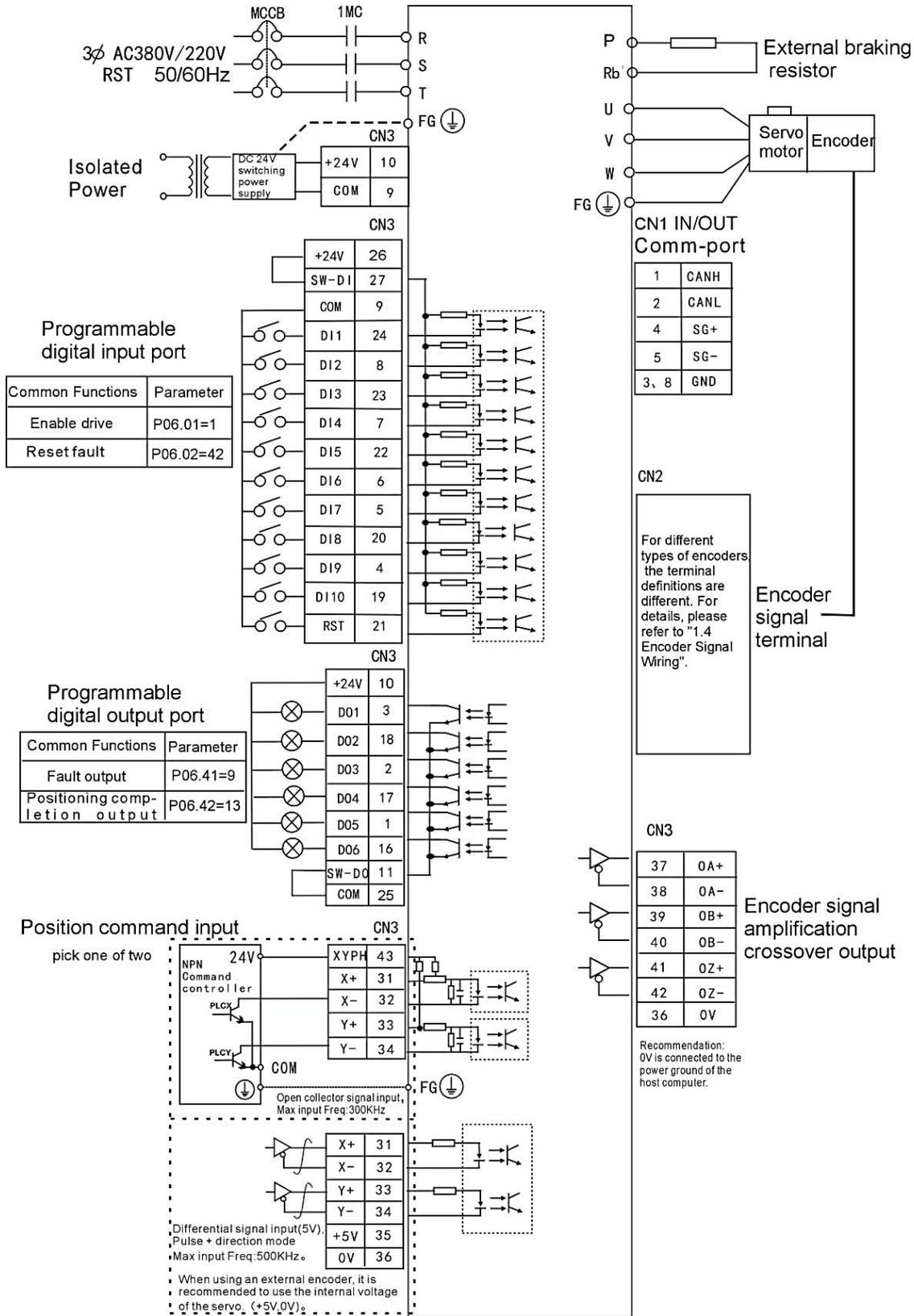
MCCB: air switch 1MC: AC contactor
