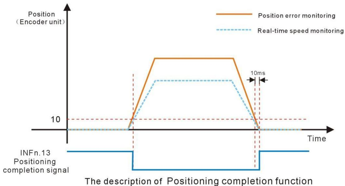
The positioning close function means that the absolute value of the position error P03.17 satisfies the condition P03.47 set by the user, and the time threshold (ms) set by P03.49 is maintained, and the positioning is considered to be close in the position control mode. At this time, the servo driver can output a positioning close signal, and the host controller receives the signal to confirm that the servo driver is positioned close.
