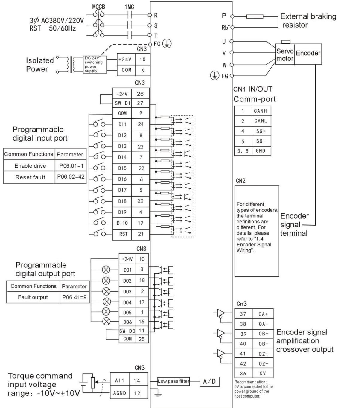
MCCB: air switch 1MC: AC contactor
