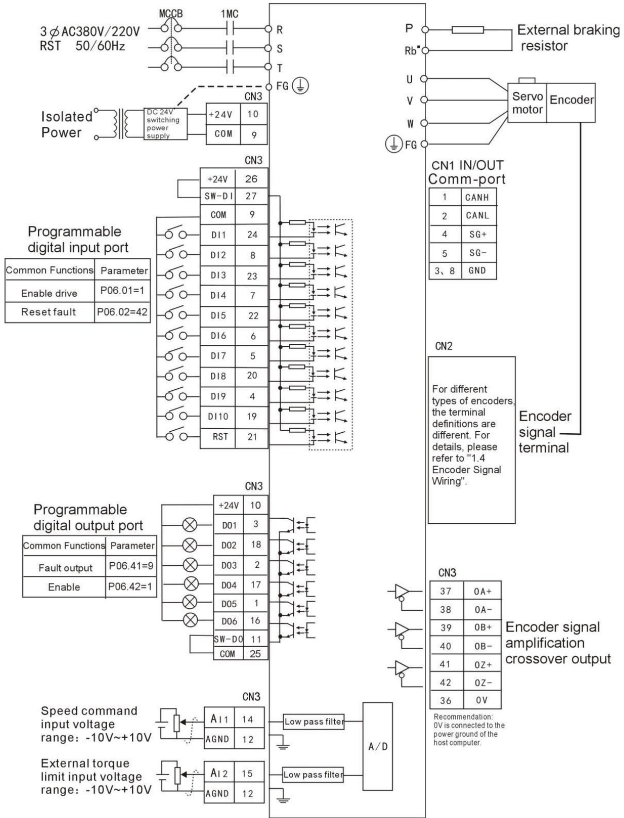
MCCB: air switch 1MC: AC contactor
