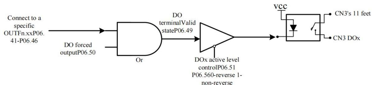
Remarks: SW-DO: Pin 11 of CN3 is short-circuited with COM for NPN mode; short-circuited with +24V is for PNP mode. For economical servo SW-DO is directly connected to COM, only NPN mode can be selected
