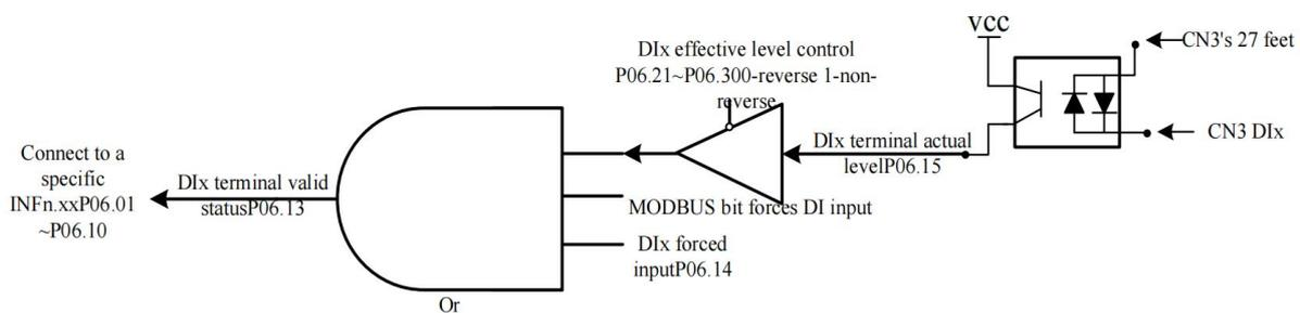
(Note: SW-DI: Pin 27 of CN3 is short-circuited with +24V for NPN mode; short-circuit with COM is for PNP mode. For economical servo SW-DI internally directly connected to 24V, only NPN mode can be selected)
