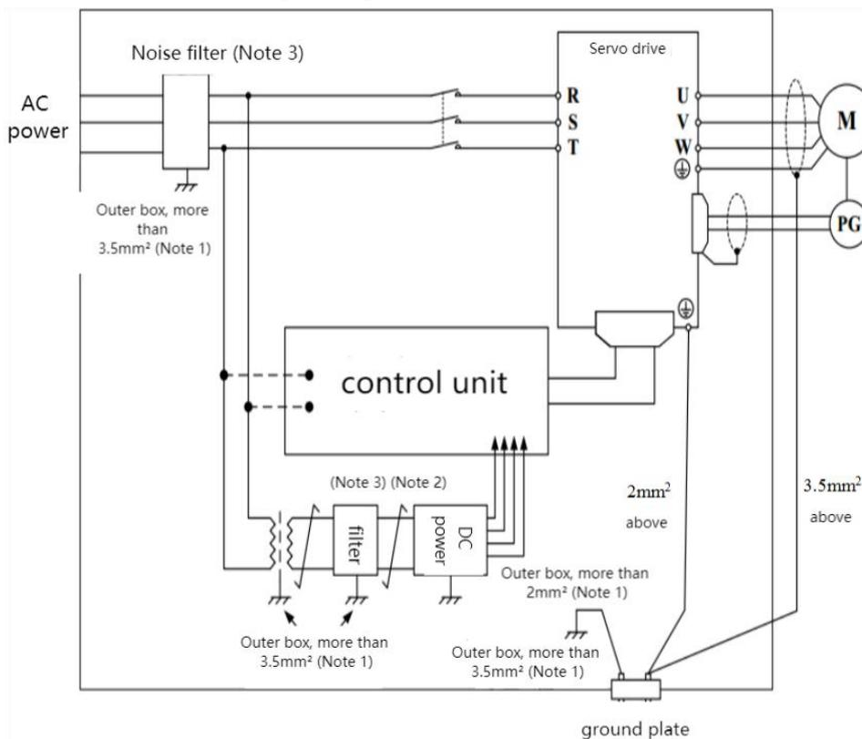
Note 1: Please use a thick wire of 3.5mm<sup>2</sup> or more for the connection wire of the outer box used for grounding (braided copper wire is recommended).
