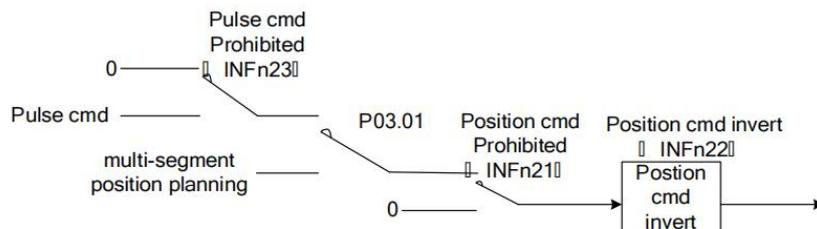
The position command can be derived from the pulse command, or from the internal multi-segment position planning, or switch between the pulse and the internal multi-segment position planning command through IO.
