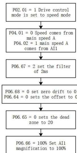
b. Take AI1 input speed command, input  $\pm 5V$  corresponding to  $\pm$  rated speed as an example:
