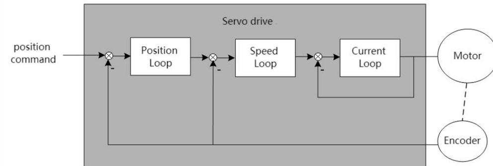
The servo driver is the control core of the servo system. By processing the input signal and feedback signal, the servo driver can control the precise position, speed and torque of the servo motor, that is, the position, speed, torque and mixed control mode. Among them, position control is the most important and most commonly used control mode of servo system.
