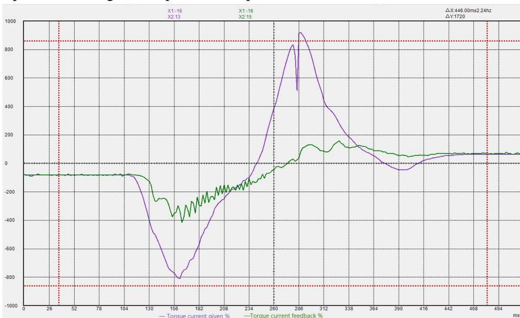
When the current loop integral gain is too large, the torque current is prone to low frequency oscillation, and overcurrent is likely to be reported during acceleration and deceleration.
