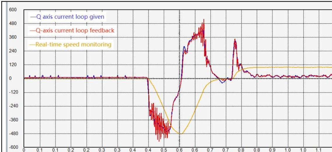
The Q-axis current has high frequency oscillation, so it is necessary to reduce the current loop proportional gain P07.01 and integral gain P07.02
