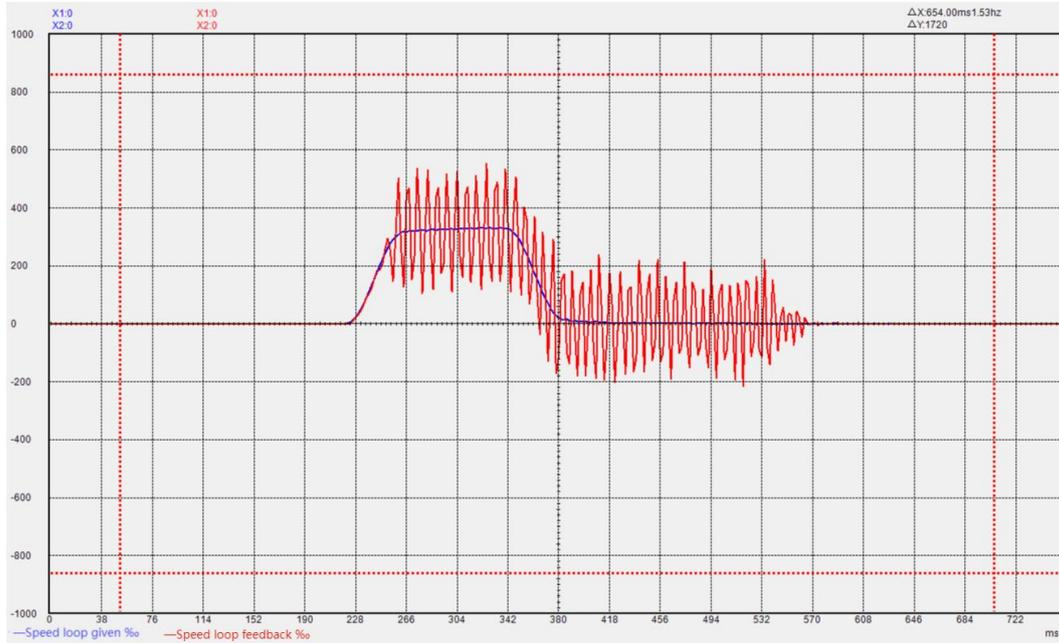
If the proportional gain of the speed loop is too small, the rigidity of the motor is very weak and the speed cannot follow.
