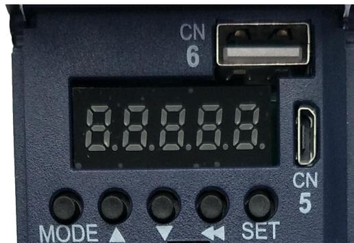
The panel contains 5 buttons and 5 digital tubes. The general functions of the 5 buttons are shown in the table below.
