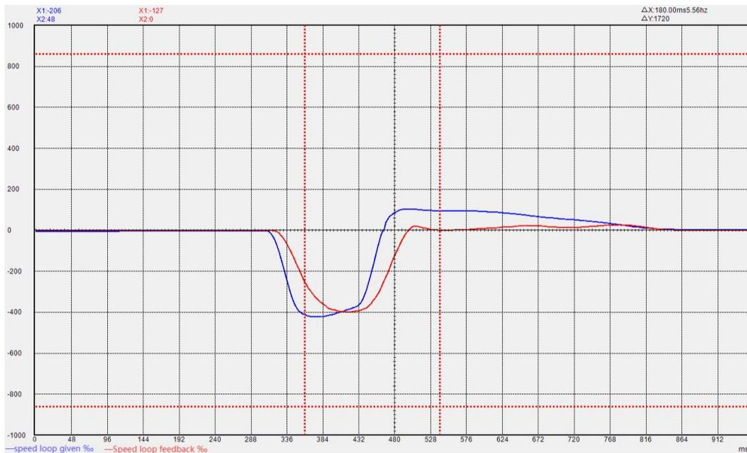
When the integral gain of the speed loop is too large, the rigidity of the motor is enhanced, and the speed is prone to low-frequency fluctuations.
