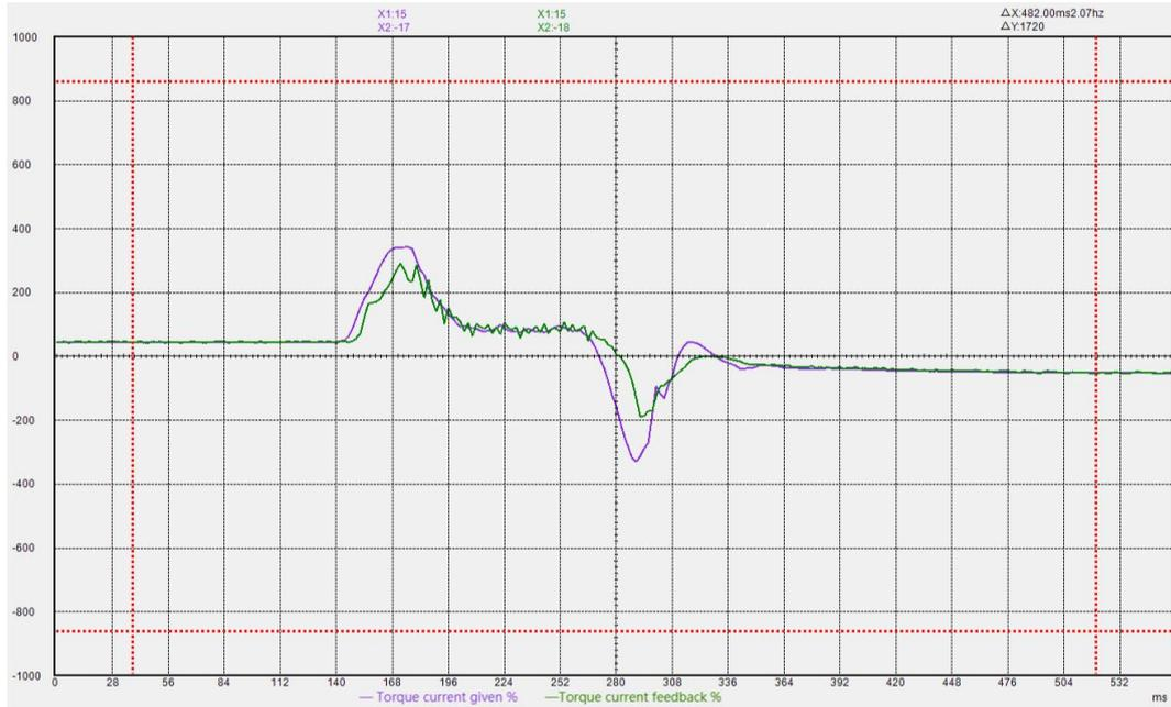
If the current loop integral gain is too small, the motor current response is slow, and the output is not enough in the process of rapid acceleration and deceleration.
