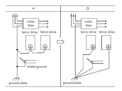
•When the noise filter and the servo drive are installed in the same control cabinet, please connect the ground wire of the noise filter and the ground wires of other devices in the control cabinet to the grounding plate of the control cabinet, and then ground.
