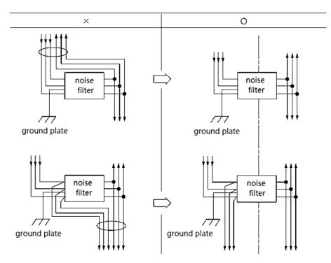
• Please separate the ground wire of the noise filter from the output wiring, do not put them in the same casing, and do not bundle them together.
