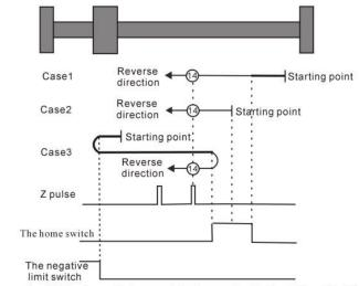
Homing method 14 Homing on the home switch, the negative limit switch and the Z index pulse
