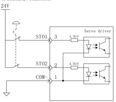
Example diagram of internal 24V connection:
