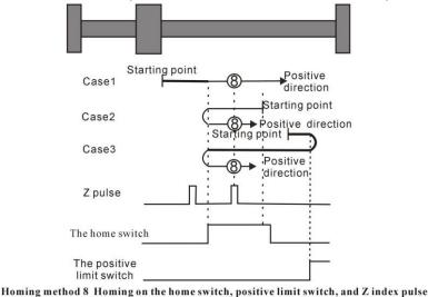
Case 1: When the user triggers the execution of homing, if the home switch state is in the low level, the axis starts to move at the first speed. When the home switch is in the high level, the motion starts at the second speed. When the switch is in the low level, the direction of motion changes and continues to move at the second speed. When the home switch is in the high level, the position where the first Z index pulse is encountered is the zero point position.
