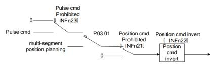
The position command can be derived from the pulse command, or from the internal multi-segment position planning, or switch between the pulse and the internal multi-segment position planning command through IO.
