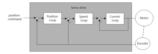
The servo driver is the control core of the servo system. By processing the input signal and feedback signal, the servo driver can control the precise position, speed and torque of the servo motor, that is, the position, speed, torque and mixed control mode. Among them, position control is the most important and most commonly used control mode of servo system.
