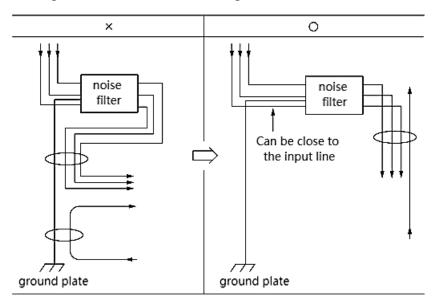
• Please connect the ground wire of the noise filter to the ground plane separately. Do not connect other ground wires.
