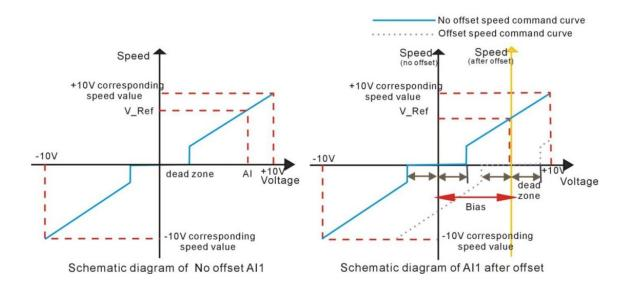
The relationship between the final speed command value percentage y6 and the input voltage x:
