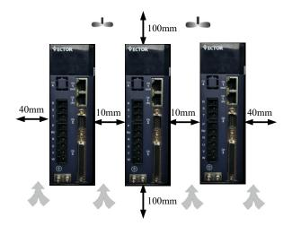
• When installing, do not block the air inlet and air outlet, and do not allow foreign objects to enter the product, otherwise it may cause malfunction or fire due to the aging of the internal components.
