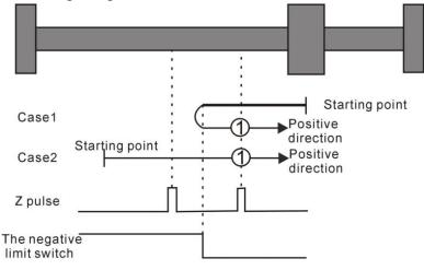
Homing method 1: Homing on the negative limit switch and Z index pulse
