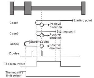
Homing method 13 Homing on the home switch, the negative limit switch and the Z index pulse
