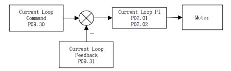
The control goal of the current loop PI is to ensure that the actual motor current (Q-axis current loop feedback) tracks the current command (Q-axis current loop given). As shown in the picture below. The Q-axis current loop feedback tracks the Q-axis current loop reference.
