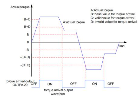
Actual torque: A; Base value for torque arrival P05.31: B; Valid value for torque arrival P05.32: C; Invalid value for torque arrival P05.33: D;
