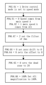
b. Take AI1 input speed command, input  $\pm 5V$  corresponding to  $\pm$  rated speed as an example:
