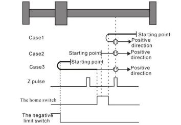
Homing method 11 Homing on the home switch, the negative limit switch and the Z index pulse
