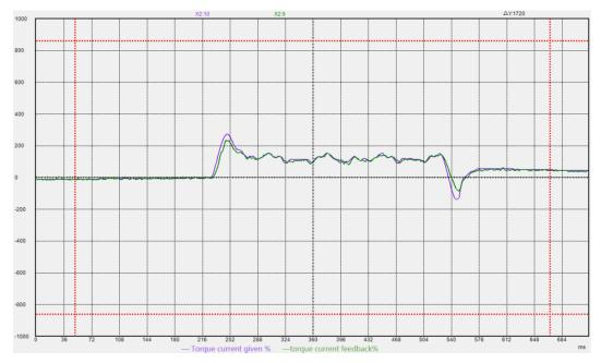
If the current loop proportional gain is too small, the motor current response is slow, and the output is not enough in the process of rapid acceleration and deceleration.
