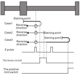
Homing method 7 Homing on the home switch, positive limit switch, and Z index pulse
