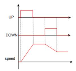
The relevant input function bits are as follows.
