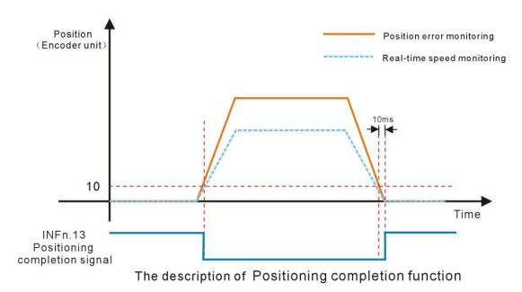
The positioning close function means that the absolute value of the position error P03.17 satisfies the condition P03.47 set by the user, and the time threshold (ms) set by P03.49 is maintained, and the positioning is considered to be close in the position control mode. At this time, the servo driver can output a positioning close signal, and the host constroller receives the signal to confirm that the servo driver is positioned close.
