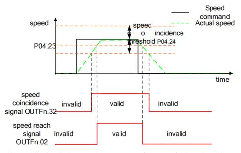
When the amplitude of the actual output speed P04.21 is less than the zero-speed threshold P04.25, the zero-speed signal OUTFn.05 is valid. When the amplitude of acceleration is greater than the acceleration threshold P04.27, the acceleration OUTFn.04 is valid. When the amplitude of the deceleration is greater than the acceleration and deceleration threshold P04.27, the deceleration OUTFn.03 is valid. The signal output is shown in the figure below.
