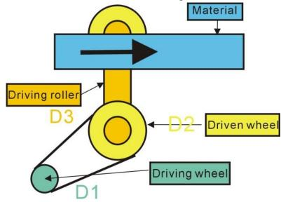
The servo motor rotates the driving wheel (diameter D1), and drives the driven wheel (diameter D2) to rotate through the belt. The transmission roller (diameter D3) and the driven wheel rotate coaxially, and at the same time drive the material to the right.
