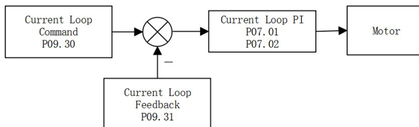
The control goal of the current loop PI is to ensure that the actual motor current (Q-axis current loop feedback) tracks the current command (Q-axis current loop given). As shown in the picture below. The Q-axis current loop feedback tracks the Q-axis current loop reference.
