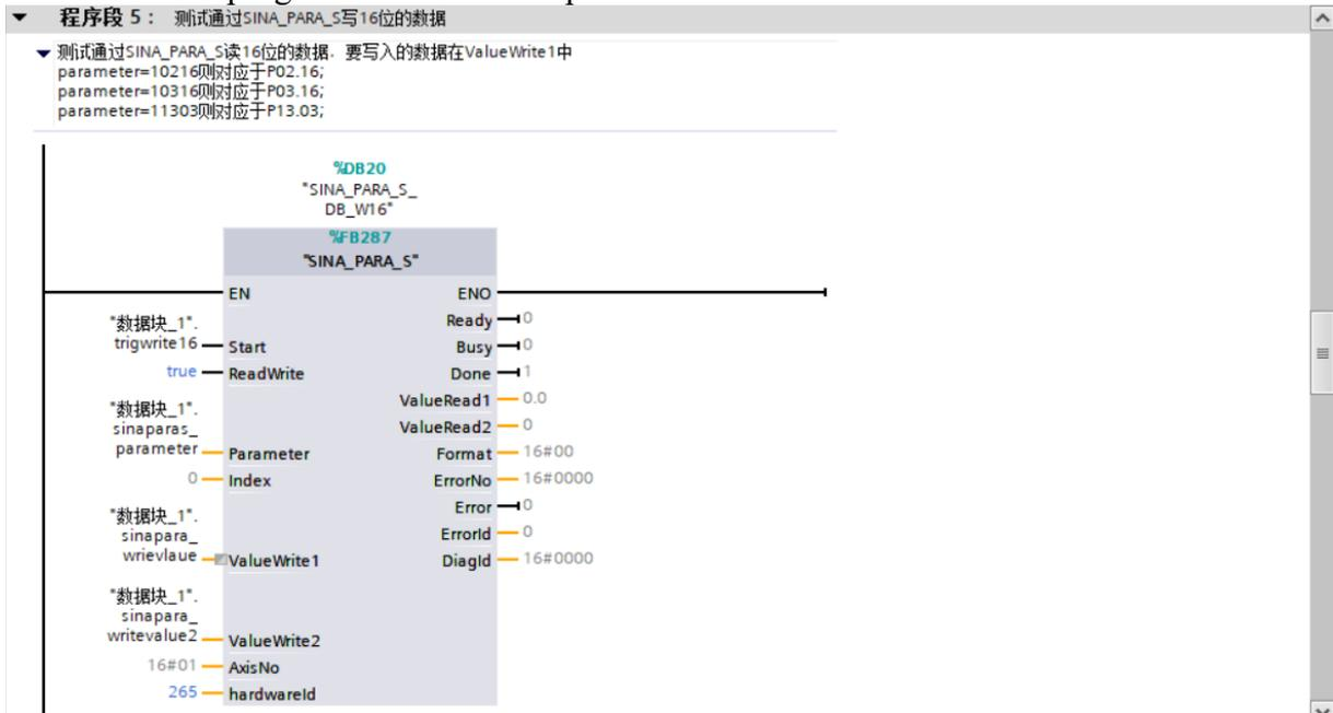
(4) The program to write 32-bit parameter data is as follows.
