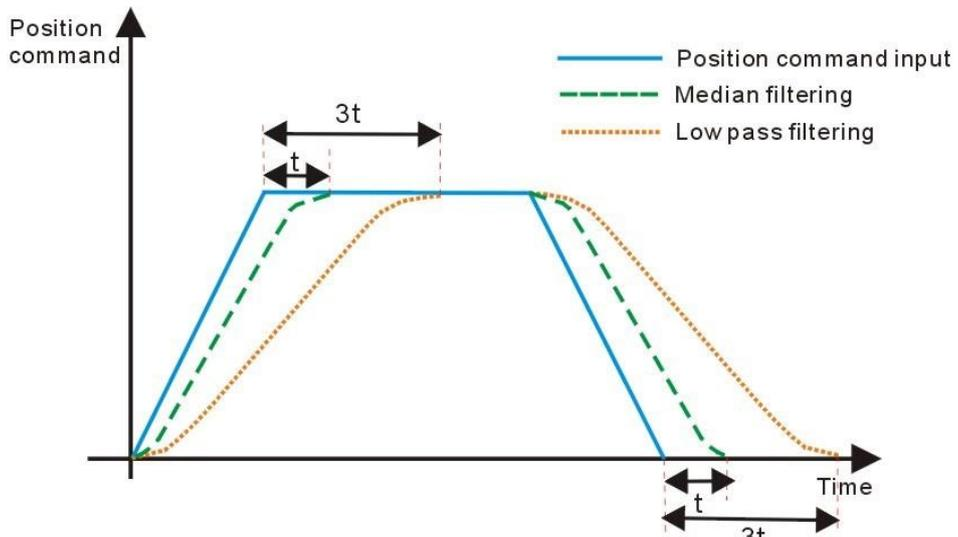
The schematic diagram of trapezoidal position command low pass filtering and median filtering
