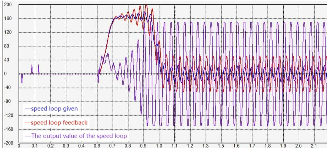
The integral gain of the speed loop is too large, the motor cannot stop all the time, and the forward and reverse rotations shake.
