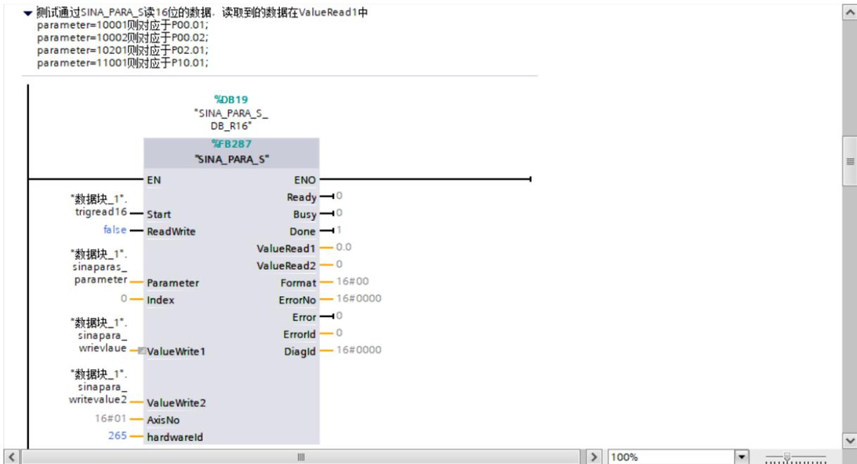
SINA\_PARA\_S The input parameters are introduced as follows.
