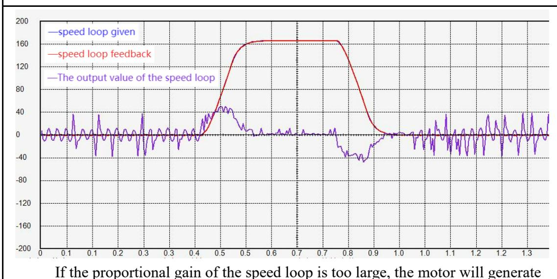
noise, and the output of the speed loop will fluctuate when it is static.
