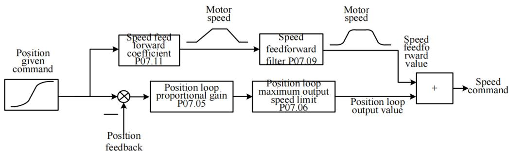
Speed feedforward refers to the mathematical operation of the given position command to obtain the speed required by the motor, which is directly given to the speed loop. As shown
