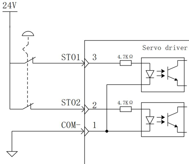
Example diagram of internal 24V connection:
