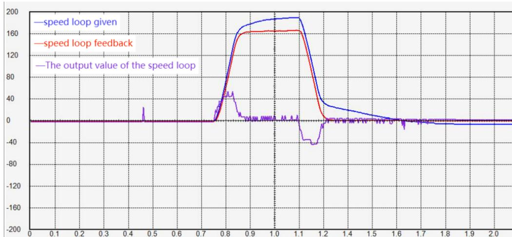
The speed loop gain is too small, the speed loop reference and feedback cannot be coincident, and the motor has no rigidity and is particularly soft.
